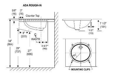
Dimensions may vary (+) or (-) 1/4". Dimensions shown in parentheses are in millimeters: 25.4 mm = 1 inch. Note: Fixture dimensions are nominal and conform with dimension and performance requirements of ASME A112.19.2-2008/CSA B45.1-08 standards. PSI rating: 20 minimum to 80 maximum per ASME A112.19.2-2008/CSA B45.1-08 standards. Dimensions subject to change or cancellation without notice. Briggs is not responsible for the use of superceded or voided specification information.
