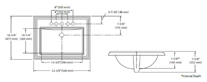
Dimensions may vary (+) or (-) 1/4". Dimensions shown in parentheses are in millimeters: 25.4 mm = 1 inch. Note: Fixture dimensions are nominal and conform with dimension and performance requirements of ASME A112.19.2-2008/CSA B45.1-08 standards. PSI rating: 20 minimum to 80 maximum per ASME A112.19.2-2008/CSA B45.1-08 standards. Dimensions subject to change or cancellation without notice. Briggs is not responsible for the use of superceded or voided specification information.
