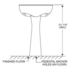
Dimensions may vary (+) or (-) 1/4". Dimensions shown in parentheses are in millimeters: 25.4 mm = 1 inch. Note: Fixture dimensions are nominal and conform with dimension and performance requirements of ASME A112.19.2-2008/CSA B45.1-08 standards. PSI rating: 20 minimum to 80 maximum per ASME A112.19.2-2008/CSA B45.1-08 standards. Dimensions subject to change or cancellation without notice. Briggs is not responsible for the use of superceded or voided specification information.
