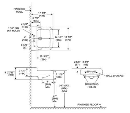
Dimensions may vary (+) or (-) 1/4". Dimensions shown in parentheses are in millimeters: 25.4 mm = 1 inch. Note: Fixture dimensions are nominal and conform with dimension and performance requirements of ASME A112.19.2-2008/CSA B45.1-08 standards. PSI rating: 20 minimum to 80 maximum per ASME A112.19.2-2008/CSA B45.1-08 standards. Dimensions subject to change or cancellation without notice. Briggs is not responsible for the use of superceded or voided specification information.
