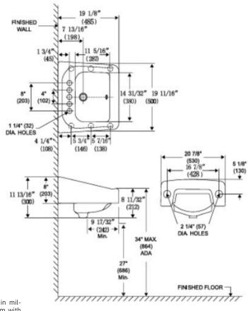
Dimensions may vary (+) or (-) 1/4". Dimensions shown in parentheses are in millimeters: 25.4 mm = 1 inch. Note: Fixture dimensions are nominal and conform with dimension and performance requirements of ASME A112.19.2-2008/CSA B45.1-08 standards. PSI rating: 20 minimum to 80 maximum per ASME A112.19.2-2008/CSA B45.1-08 standards. Dimensions subject to change or cancellation without notice. Briggs is not responsible for the use of superceded or voided specification information.
