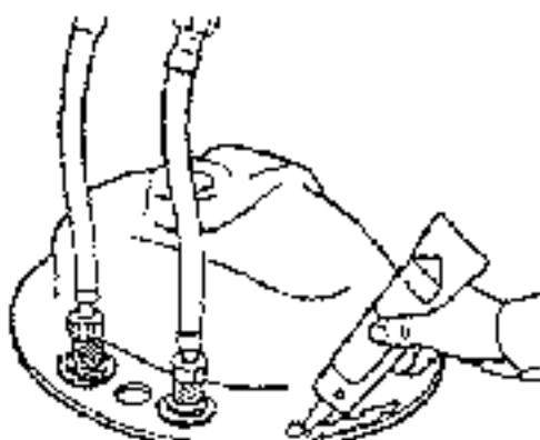
Squeeze a bead of sealant 1/4" from edge.
